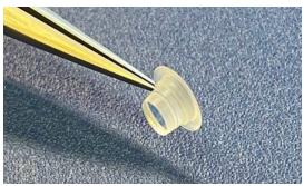
• The front plate is a solid piece of PMMA with a mushroom shape, with an anterior lip (5.0 mm in diameter), and stem (3.35 mm in diameter). (one/pouch)
